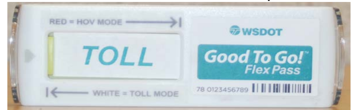
Driver shifts transponder window left for Toll Mode (WHITE)
