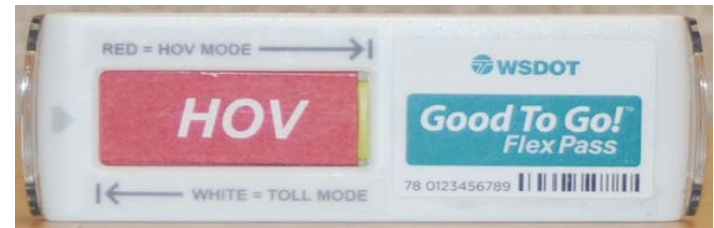
Driver shifts transponder window right for HOV Mode (RED)
